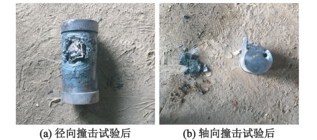
图 4 12.7 mm 子弹撞击试验后 CL-20 基压装型温压炸药的状态 Fig. 4 Experimental states of CL-20 based pressed thermobaric explosive after 12.7 mm bullet impact test
