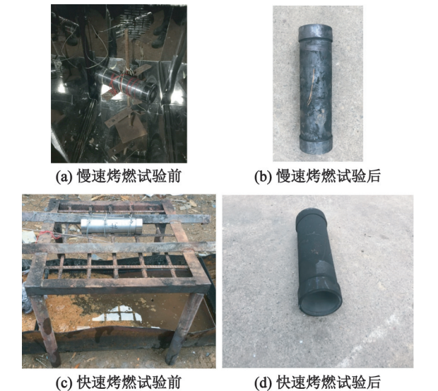
图 3 烤燃试验前、后 CL-20 基压装型温压炸药的状态 Fig. 3 Experimental states of CL-20 based pressed thermobaric explosive before and after fast or slow cook-off tests
