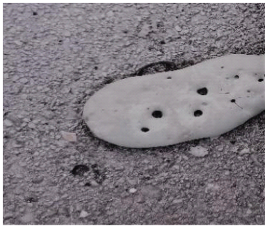
图 4 氧差为 0 时的残渣 Fig.4 Residue when oxygen difference is 0
