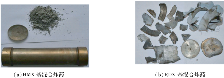
图6 两种炸药慢速烤燃试验结果 Fig. 6 Slow cook-off test results of the two explosives
