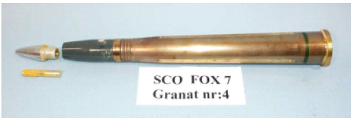
图 9 慢速烤燃试验结果 Fig.9 Results of slow cook-off test
