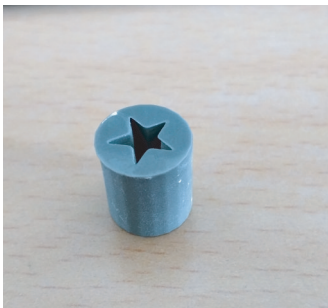
图 6 3D 打印推进剂药柱 Fig. 6 3D-printed propellant grain
