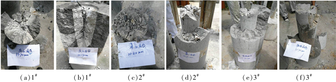
图 4 碳酸盐岩地面打靶试验结果 Fig.4 Ground target test results of carbonate rock
