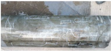
图 1 磨损失效轧辊初次爆炸焊接实验 Fig.1 The preliminary explosion welding experiment for worn roller
