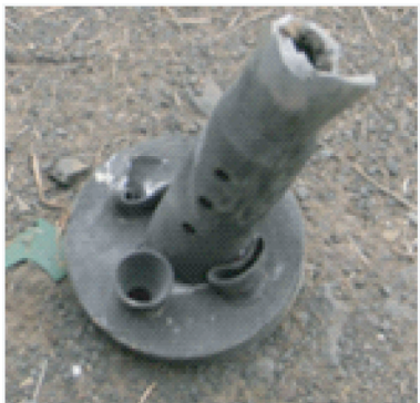
图 12 被拦截后的破甲弹 Fig. 12 High explosive anti-tank cartridge after being intercepted
