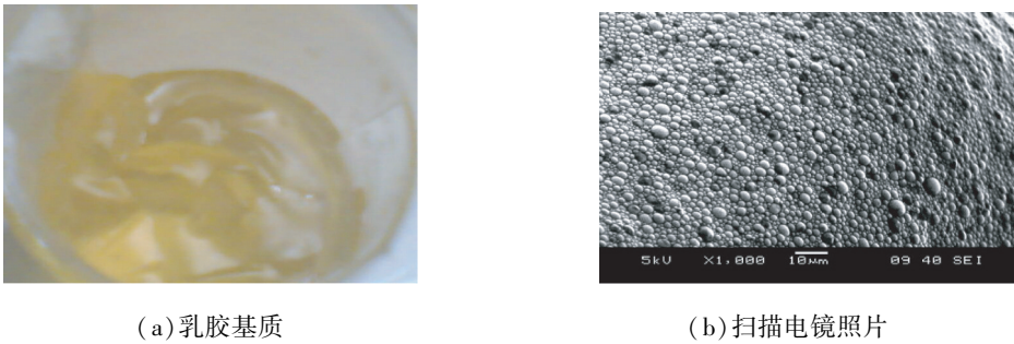
图3 乳胶基质及其扫描电镜照片 Fig.3 Emulsion matrix and its SEM photos
