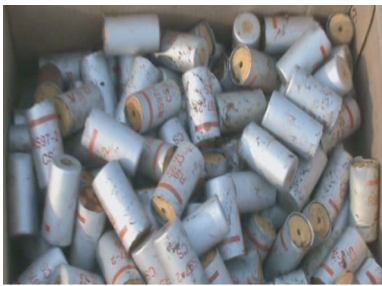
Fig. 2 Cutting example of anti-riot ammunitions
