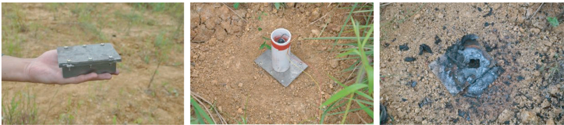
图 3 高能燃烧剂销毁模拟地雷 Fig. 3 Simulated mine destroyed by termite
