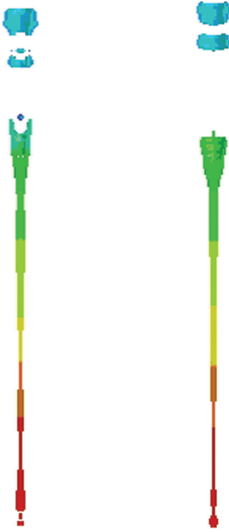
(a) 垂直侵彻 ERA (b) 未侵彻 ERA 图 5 100 \mu\text{s} 时侵彻体形态对比 Fig.5 Comparison of the shape of the penetrating body at 100 \mu\text{s}
