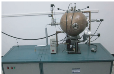
图 1 特殊环境 20 L 爆炸特性测试系统的主要部分 Fig.1 The main part of 20 L explosion characteristic test system in extraordinary circumstance
