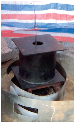
图3 烤燃试验装置 Fig.3 Device of Baking test
