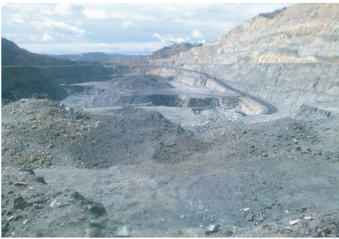
图 5 ▽ 2#1058 平台爆破效果(左原配方,右试验配方) Fig. 5 Blasting effect of ▽ 2#1058 platform (the original recipe on left, the test recipe on right)
